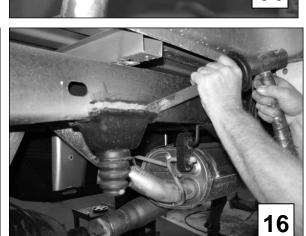
7c) Use an abrasive grinder to remove the excess material on the frame once the bracket has been removed. Use black spray paint to protect the raw exposed metal.
